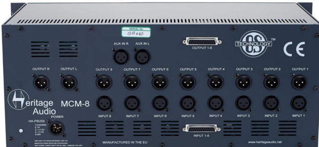
Upper row on the back panel corresponds to the individual XLR and combined DSUB channel outputs.
